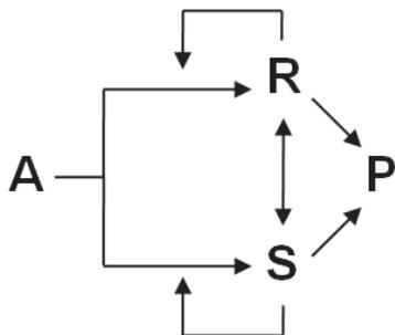
Fig. 2: Sketch of the chemical model indicating two autocatalytic feedback loops involved in the formation of the chiral products  $R$  and  $S$  from the achiral substrate  $A$  ( $A + R \rightarrow 2R$ ,  $A + S \rightarrow 2S$ ), the racemization of the enantiomers ( $R \rightleftharpoons S$ ) and a cross-inhibition between them yielding an inactive product  $P$  ( $R + S \rightarrow P$ ).
