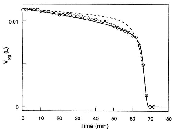
Fig. 3. Kinetics of ethyl hexanoate biphasic hydrolysis.  $\circ\circ\circ$ : experimental points; ----: best fit obtained with the model used in Section 3.2 implying only one size aggregates; —: best fit obtained with the model implying two sizes aggregates.
