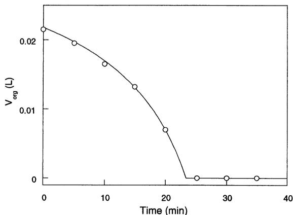
Fig. 1. Volume of the organic phase as a function of time in the biphasic hydrolysis of ethyl butanoate using  $3 \text{ mol l}^{-1}$  NaOH aqueous solution.  $T = 60^\circ\text{C}$ ,  $V_{\text{org}0}/V_{\text{tot}} = 22\%$ , stirring rate: 800 rpm.  $\circ\circ\circ$ : experimental points; —: simulation.
