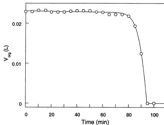
Fig. 2. Volume of the organic phase as a function of time in the biphasic hydrolysis of ethyl octanoate using  $3 \text{ mol l}^{-1}$  NaOH aqueous solution.  $T = 80^\circ\text{C}$ ,  $V_{org0}/V_{tot} = 22\%$ , stirring rate: 800 rpm.  $\circ\circ\circ$ : experimental points; —: simulation.
