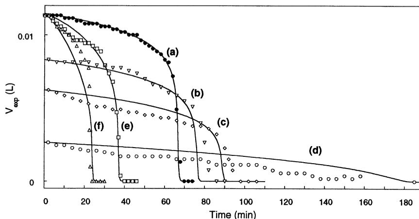
Fig. 4. Kinetics of ethyl hexanoate biphasic hydrolysis. A: effect of initial ester volumes: (a)  $V_{org0} = 11.5$  ml (0.069 mol); (b)  $V_{org0} = 8.5$  ml (0.051 mol); (c)  $V_{org0} = 6.5$  ml (0.039 mol); (d)  $V_{org0} = 3$  ml (0.018 mol). Stirring rate is 600 rpm in each case. B: effect of stirring rate: (a) 600 rpm (this experiment is common to both series); (e) 800 rpm; (f) 1050 rpm ( $V_{aq0} = 38.5$  ml for all the experiments). —: simulations.)
