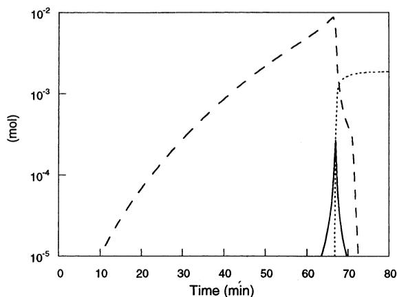
Fig. 5. Concentration profiles obtained from simulation of experimental curve represented in Fig. 3. Dashed line: ECA<sub>1</sub>; solid line: ECA<sub>2</sub>; dotted line: M.
