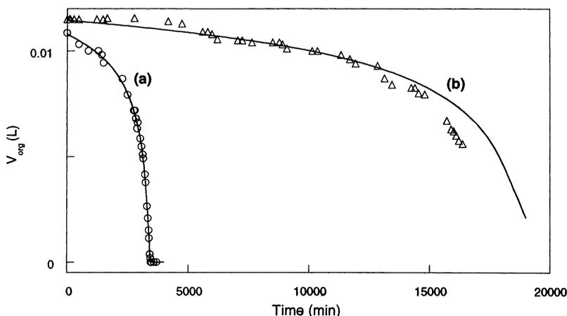
Fig. 6. Non-emulsified reaction: (a) cross section surface is  $18.9 \text{ cm}^2$  (fitted); (b) cross section surface is  $3.3 \text{ cm}^2$  (predicted using parameters obtained for curve (a)).  $\circ\circ\circ$ : experience, —: simulation.
